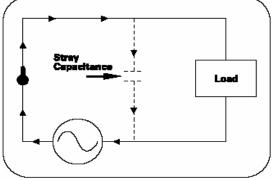
Also, if an arc-suppression capacitor is used across the contacts, this capacitance will discharge itself through the relay contacts.
