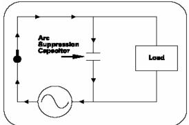
The discharge surge current may be hundreds of amperes for a few nanoseconds or more. To limit such discharge currents, an arc suppression capacitor should have a certain amount of resistance in series with it. In circuits where there is no dedicated capacitance, however, there still may be sufficient stray capacitance to cause a momentary over current upon contact make. This fact is often overlooked by many circuit designers.
