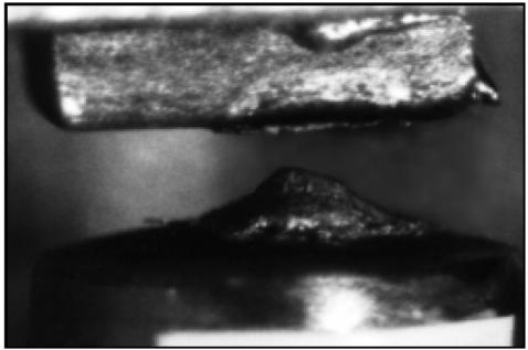
Another result of severe arcing which may occur now and then is contact welding. Usually, though, when this happens, it is evidence that the relay has been misapplied in a circuit where voltage and/or current are much greater than that particular relay can handle.
